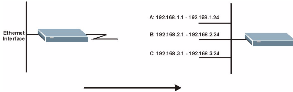
Figure 15 Physical Network & Partitioned Logical Networks
